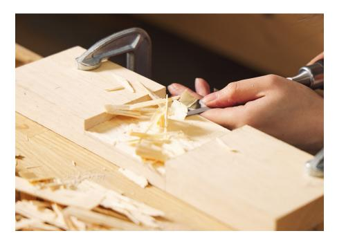
**Tip:** Cut down to the baseline by paring across the grain, cutting about halfway across the width of the piece. If you cut all the way across the workpiece, there is a chance that you will experience tear-out. That is, the wood will tear ahead of the chisel's cutting edge. Pay attention to the direction of the grain; you may need to take slightly angled cuts in the direction of the grain if it runs out.
