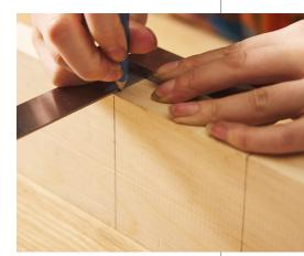
g. To lay out the depth of the joint, measure and mark 1/2" down from the face along each shoulder line. Draw a line to connect these two points. Do this on both edges.
