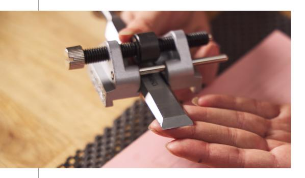
h. The final step is to remove the burr on the face of the chisel blade. Apply a bit of water onto the 3 micron film, place the face of the chisel flat on the film and take a couple of lapping strokes to remove the burr.
