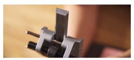
g. The third step in sharpening a chisel blade is to polish the secondary bevel. Switch to the 3 micron side of the sharpening block. Draw the guide and chisel toward you a few times. Once you're satisfied there is an even polish across the blade's edge, remove the chisel from the guide.
