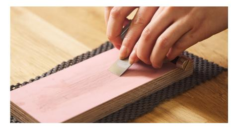
e. If the 9 micron film is worn from lapping, replace it with a fresh piece.
