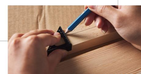
e. Place the square flush with the short edge of the front piece. Measure and make a pencil mark 1" inset from one end. Turn the square 90° and extend the line. Place the square on the other short edge, measure and mark 1" inset from that end, then extend the line.
