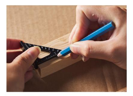
f. To mark the center between the 3/4" reference line and the bottom edge of the front piece, place the square flush with the long edge and near the 1" inset mark and draw a line 3/8" up from the bottom edge. Make another 3/8" mark on the other end. Align the ruler with both marks and draw a line to cross the 1" and 4 5/8" lines.
