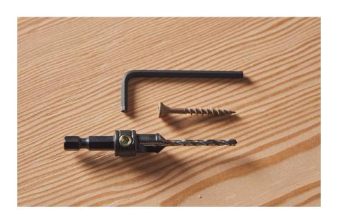
i. Adjust the projection of the 1/8" drill bit within the #8 countersink as required for the deck screw. (For the 1 1/2" long deck screws, the drill bit should project about 1".) Install the countersink bit in a hand drill.
