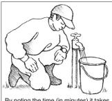
By noting the time (in minutes) it takes to fill a 5-gallon pail, gallons per hour (gph) can be calculated: 60 ÷ number of minutes x 5 = "x" gph.
